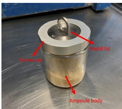
Figure 5.2. 125 mL glass ampoule (Photograph taken on 15 December 2023).
