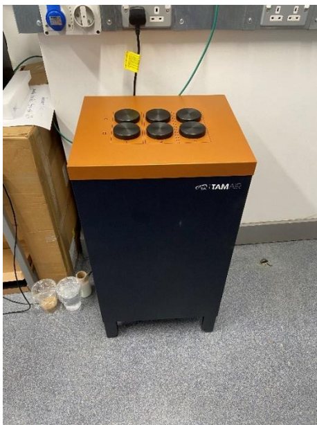
Figure 5.1. TAM Air 3-channel isothermal calorimeter (Photograph taken on 02 February 2023).
