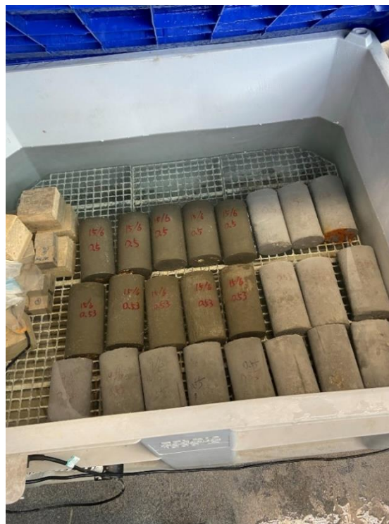
Figure 3.1. Cylinder specimens in the 20°C-water bath (Photograph taken on 29 April 2022).
