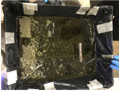
(a) FRP in the resin bath
