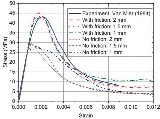
Fig. 7. Stress-strain curves of the uniaxial compression test
