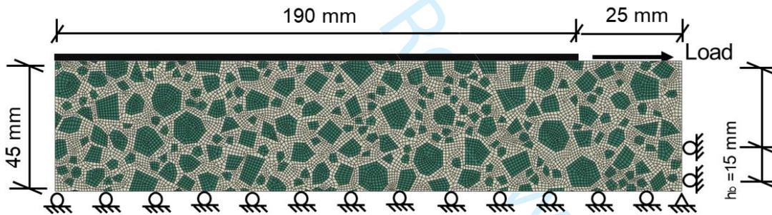
Fig. 10. 2D *meso-scale* FE model of an FRP-to-bonded joint under single shear
