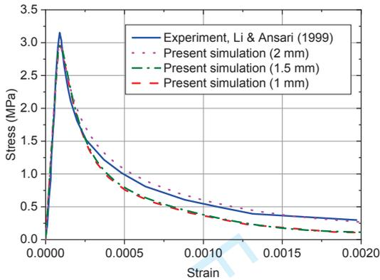
Fig. 3. Stress-strain curves of the uniaxial tension test
