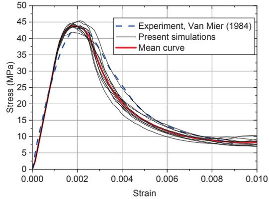
Fig. 8. Stress-strain curves for 10 samples of the uniaxial compression test with end friction
