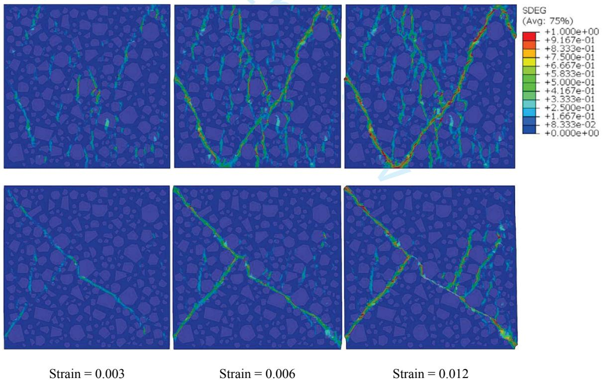
Fig. 9. Effect of boundary friction on uniaxial compression (top row: no friction; bottom row: friction coefficient = 0.47)
