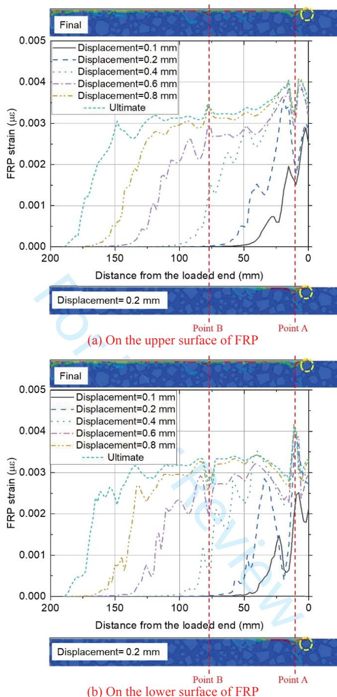
Fig. 14. Strain distributions at different loading levels of specimen II-5 in Yao *et al.* (2005)
