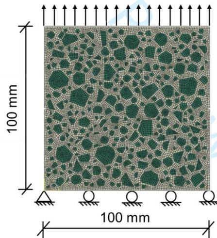
Fig. 2. A *meso-scale* numerical model under uniaxial tension
