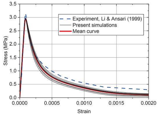
Fig. 4. Stress-strain curves for 10 samples of the uniaxial tension test
