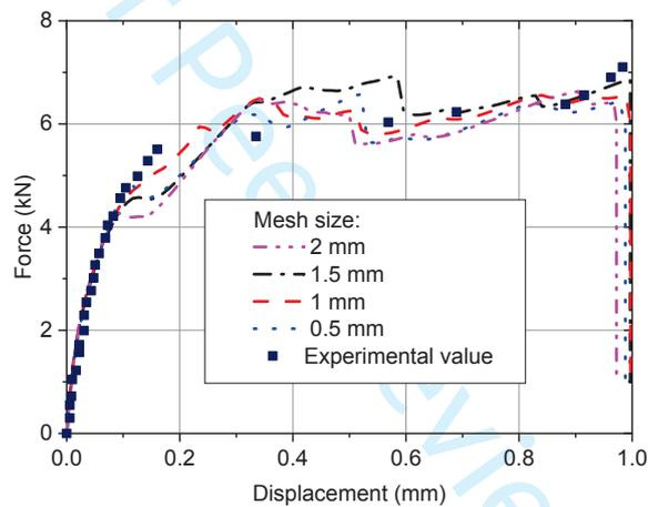
Fig. 11. Load-displacement curves of the single shear test
