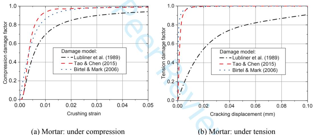
Fig. 16. Damage evolution curves of three models for the mortar (1 mm element size)
