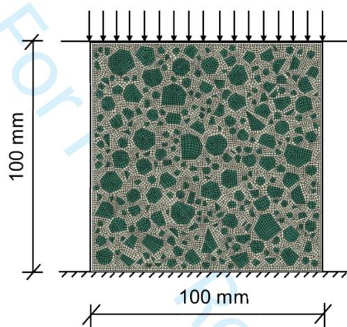
Fig. 6. A meso-scale numerical sample under uniaxial compression
