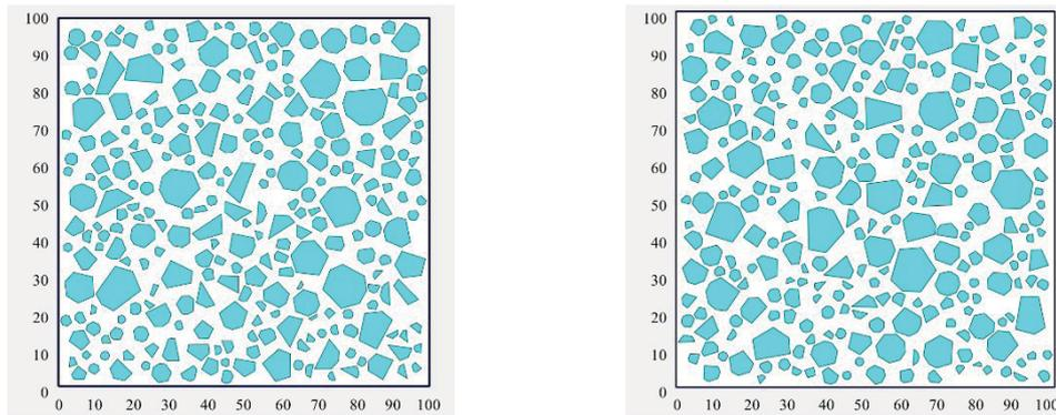
Fig. 1. Computer generated 100 mm square meso-scale concrete samples
