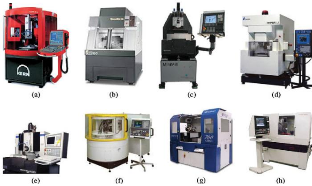
Figure 2.7 Industrial precision machine tools with micro cutting capability[2]: a) Kern micro; b) Sodick AZ15; c) Fraunhofer IPT Minimill; d) Makino Hyper 2J; e) Kuglar MicroMaster MM2; f) Fanuc ROBOnano; g) Precitech freeform 700 Ultra; h) Moore Nanotech 350FG.
