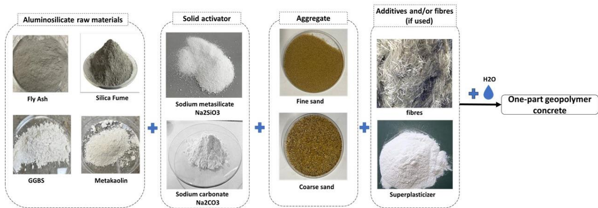
Figure 2.1. One-part AAM preparation for 3D printing application [61]
