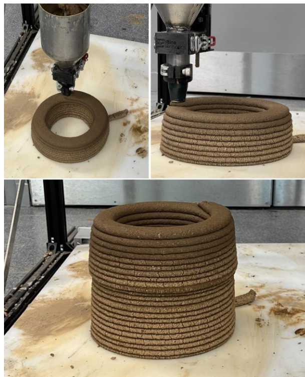
Figure 5.13. Buildability performance of the M-1S-0.6VMA mixture
