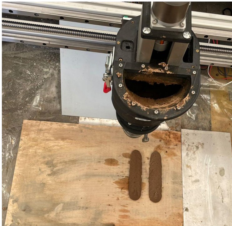
Figure 4.7. Straight lines extruded to assess the open time of the mixture.
