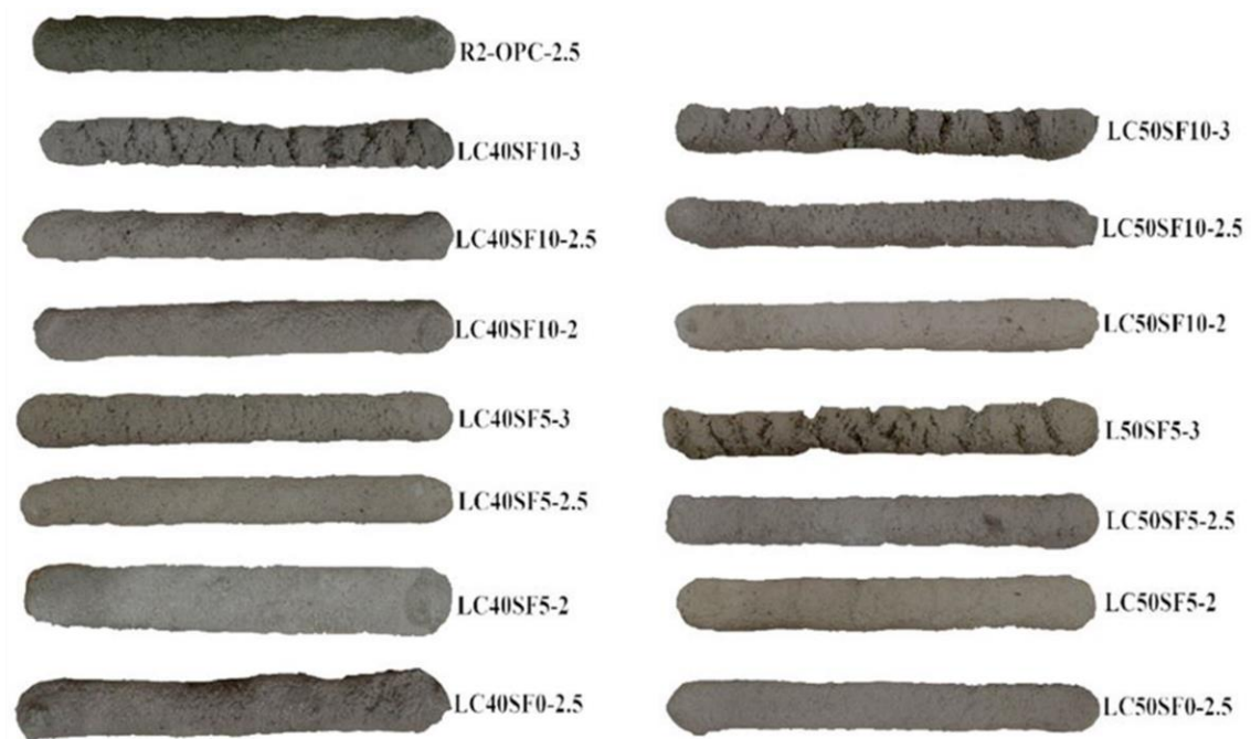
Figure 2.14. Extrudability of LC3 mixtures with different limestone-calcined clay, SF and sand contents [185]
