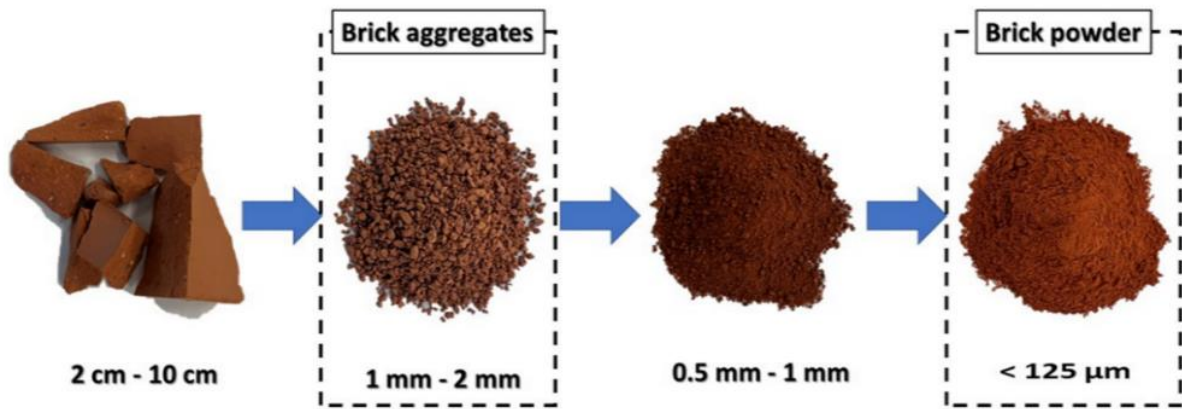
Figure 3.3. Brick powder and brick aggregate preparation process.
