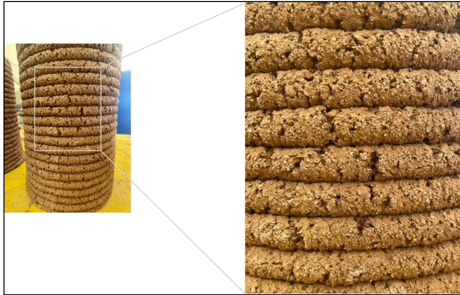
Figure 6.13. Layers' printing quality of LC3-50BA mix.
