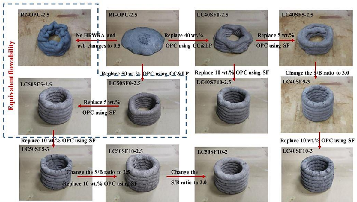
Figure 2.17. Buildability and shape retention of the object using different LC3 mix formulations [185]
