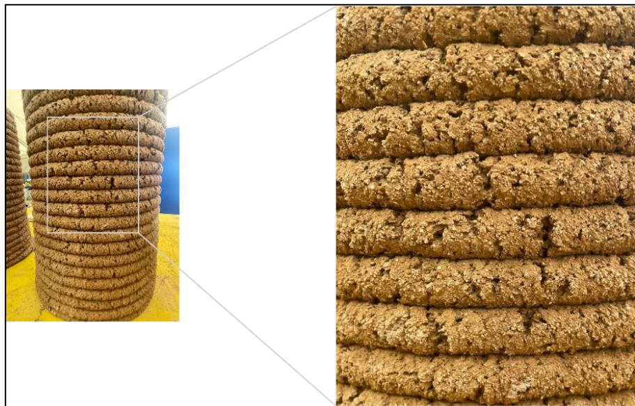
Figure 6.12. Layers' printing quality of LC3-30BA mix.
