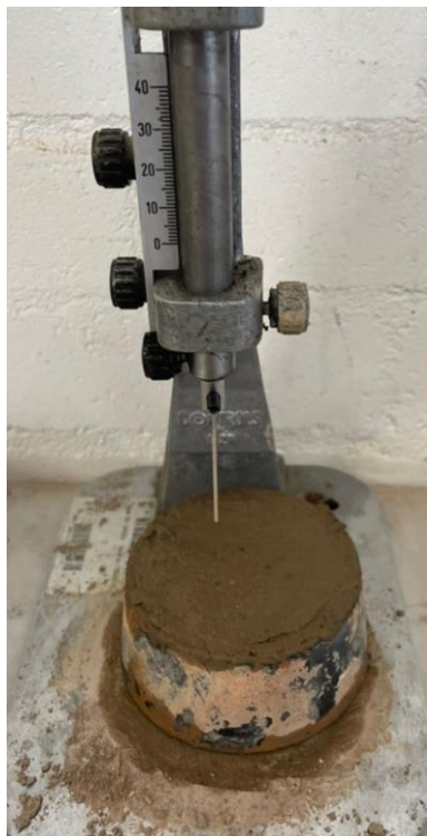
Figure 4.6. Vicat apparatus and the cone for setting time assessment.
