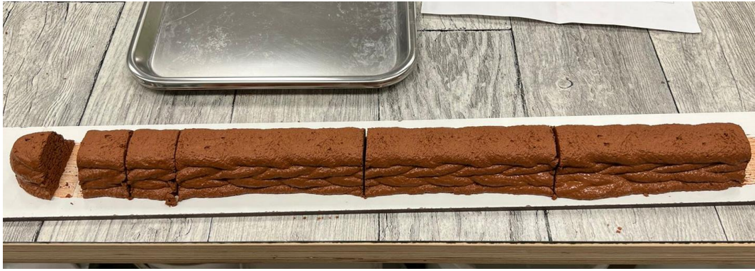
Figure 4.5. 3D printed line cut into prismatic samples for mechanical properties.
