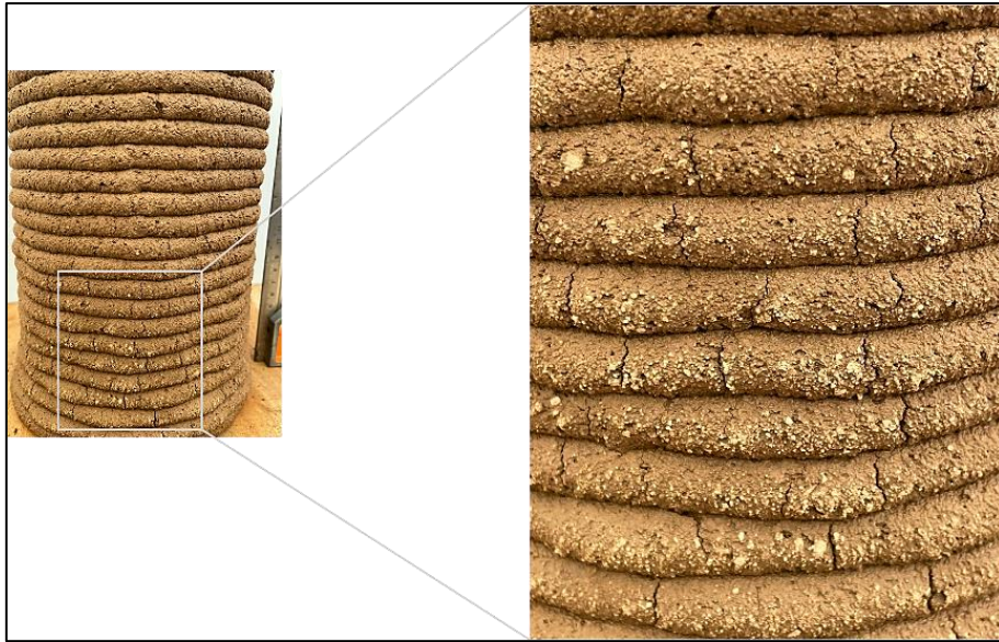
Figure 6.11. Layers' printing quality of LC3 with NA (CS mix).
