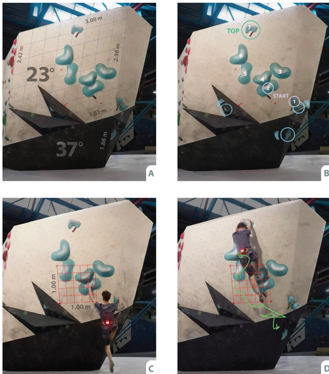
FIGURE 1 | Visual representation of the variability test set-up: (A) The wall angles and dimensions. The blue rectangular grid was placed over the main panel of the wall to show there is only very limited lens distortion after the Linear FOV correction (i.e., grid and upper and lower edges of the wall are largely aligned). (B) In light-blue the starting holds, the top holds, seven hand holds, three footholds and two volumes; (C) The (red) perspective grid, connecting three markers in horizontal and vertical position in the centre of the wall, that was used to define a coordinate system in the plane of the wall for the x - and y -position of the marker in terms of real-world coordinates. The participant is situated in the starting position here, with the light bulb attached to the back being selected as a marker for semi-automated tracking in Kinovea. (D) An example of a hip trajectory from a successful attempt on the variability test, tracked by Kinovea and expressed relative to the (red) perspective grid.
