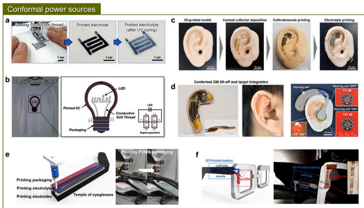
Fig. 22. Conformal power sources. a) Fabrication process of stencil-printed SC on T-shirts. b) Photograph of wearable electronic garments featuring SCs designed as a bulb symbol capable of operating LEDs. Reproduced from Ref. [325] with permission from Wiley-VCH GmbH, Copyright 2018. c) Photographs depicting the sequential fabrication and integration of conformal ZIB with human ear. d) Photograph of ear-shaped conformal ZIB connected to hearing aid connected with an LED, demonstrating successful operation of the LED and amplifier by the conformal ZIB. Reproduced from Ref. [307] with permission from Wiley-VCH GmbH, Copyright 2023. e) Schematic and photo images of a 3D DIW-printed LIB with packaging on an eyeglasses temple. f) Photographs of fabricated conformal printed battery onto 3D eyeglasses, powering connected micro-LEDs. Reproduced from Ref. [355] with permission from Elsevier, Copyright 2023.
