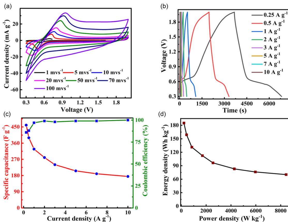
**Figure 9.** a) CV at various scan rates, b) GCD at various current densities, c) specific capacitance and coulombic efficiency as a function of different current densities, and d) Ragone plot of ZIC with 3 mM ChAQs/1.8 M ChCl/1 M ZnCl<sub>2</sub> electrolyte system.
