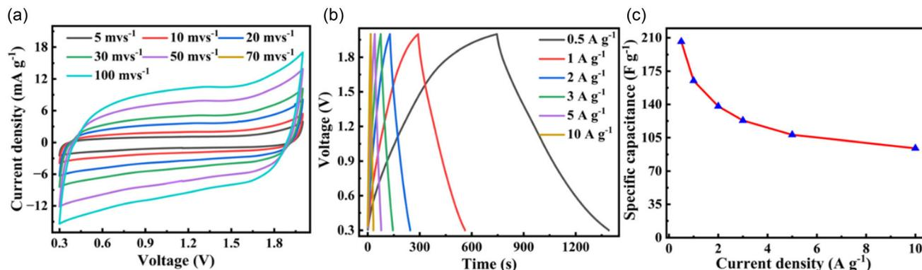
**Figure 6.** a) CV curve at different scan rates, b) GCD at different current densities, and c)  $C_{s,2E}$  as a function of current densities of ZIC in 1.8 M ChCl/1 M ZnCl<sub>2</sub> electrolyte.
