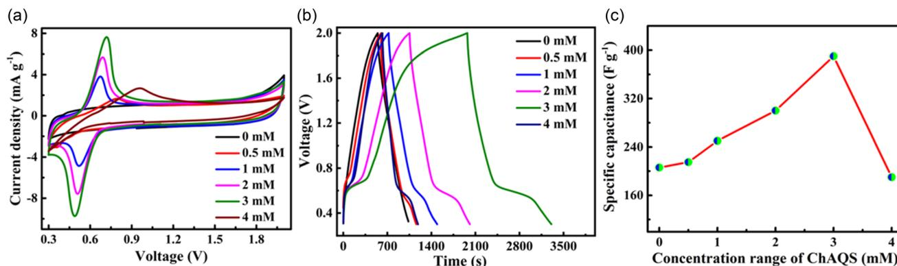
**Figure 7.** a) CV curve at different scan rates, b) GCD at different current densities, and c)  $C_{S,2E}$  as a function of current densities of ZIC in x mM ChAQS/1.8 M ChCl/1 M ZnCl<sub>2</sub> electrolyte.
