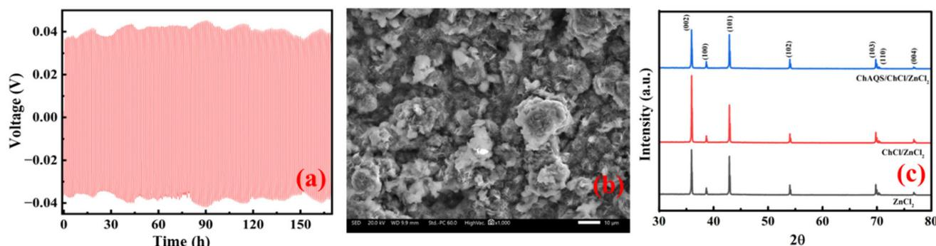
**Figure 8.** a) The Zn plating/stripping in a Zn/Zn symmetric cell with 3 mM ChAQS/1.8 M ChCl/1 M ZnCl<sub>2</sub> electrolyte at 2 mA cm<sup>2</sup> with a sweep duration of 10 min over 180 h, b) SEM images of the Zn electrodes after cycling, and c) XRD spectra of the Zn electrode after long-term galvanostatic testing in electrolytes of ZnCl<sub>2</sub>, ZnCl<sub>2</sub>/ChCl, and ChAQS/ChCl/ZnCl<sub>2</sub>.
