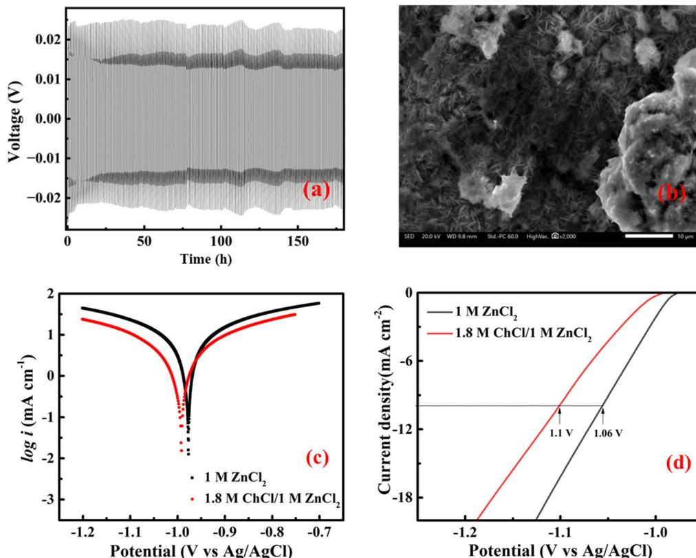
**Figure 4.** a) The Zn plating/stripping in a Zn/Zn symmetric cell with  $1.8 \text{ M ChCl}/1 \text{ M ZnCl}_2$  electrolyte at  $2 \text{ mA cm}^{-2}$  with a sweep duration of 10 min over 180 h, b) SEM image of Zn electrodes after cycling, c) corrosion curves of Zn electrode, and d) LSV curves of Zn electrode in  $\text{ZnCl}_2$  and  $\text{ChCl}/\text{ZnCl}_2$  electrolyte.
