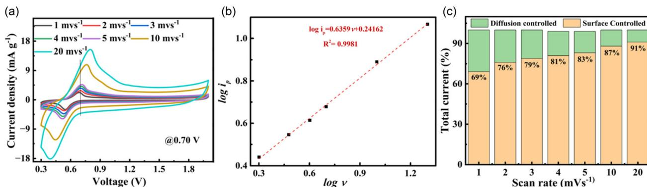
**Figure 10.** a) CV curves of the graphene/Zn electrode at various scan rates ranging from 1 to 20 mV s<sup>-1</sup> in the electrolyte of 3 mM ChAQs/1.8 M ChCl/1 M ZnCl<sub>2</sub> electrolyte system, b)  $\log(i_p)$  versus  $\log(v)$  curves relationship for peak as shown in Figure 4a, and c) capacity contribution ratio at various scan rates from 1 to 20 mV s<sup>-1</sup>.
