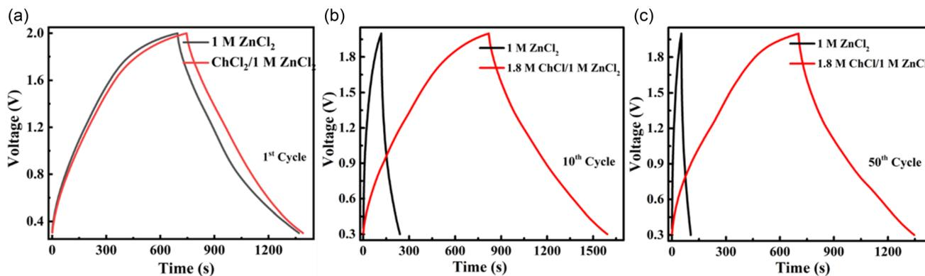
**Figure 5.** GCD curves at a current density of 0.5 A g<sup>-1</sup> for ZIC device with 1.8 M ChCl/1 M ZnCl<sub>2</sub> and 1 M ZnCl<sub>2</sub> a) 1st cycle, b) 10th cycle, and c) 50th cycle.
