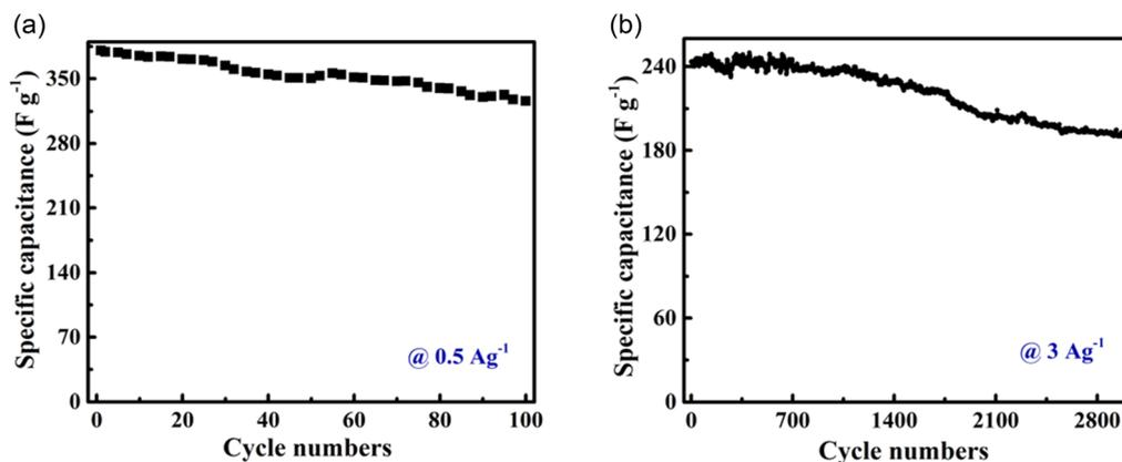
Figure 11. The stability curve for ZIC with 3 mM ChAQS/1.8 M ChCl/1 M ZnCl<sub>2</sub> at a current density of a) 0.5 A g<sup>-1</sup>, and b) 3 A g<sup>-1</sup>.
