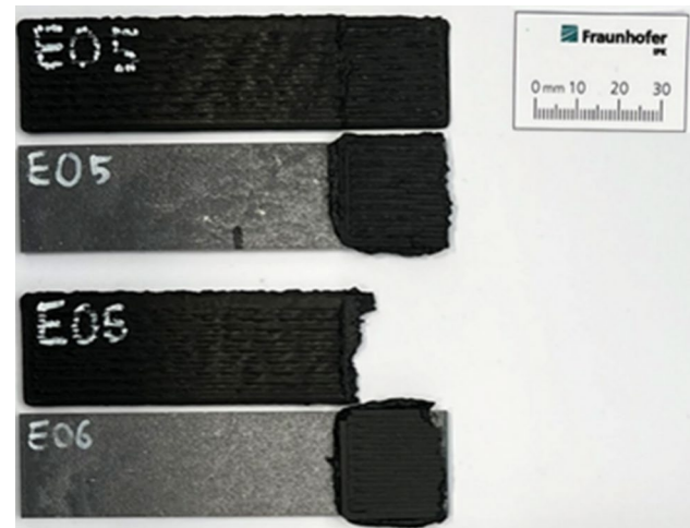
Fig. 5 Image of fracture patterns of test coupons after the lap-shear test
