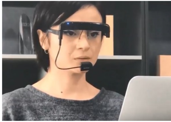
Figure 2. Head mouse, controlling the mouse by head movement. ( https://www.assistivetechlogyservices.com/headmouse.html ).
