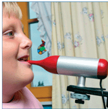
Figure 3. Integra mouse, operated via suck and puff ( https://www.mkprosopsis.com/hardware/IntegraMouse.htm ).
