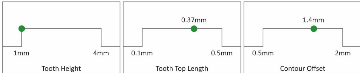
Figure 77. Optimal parameters for contour-type supports.
