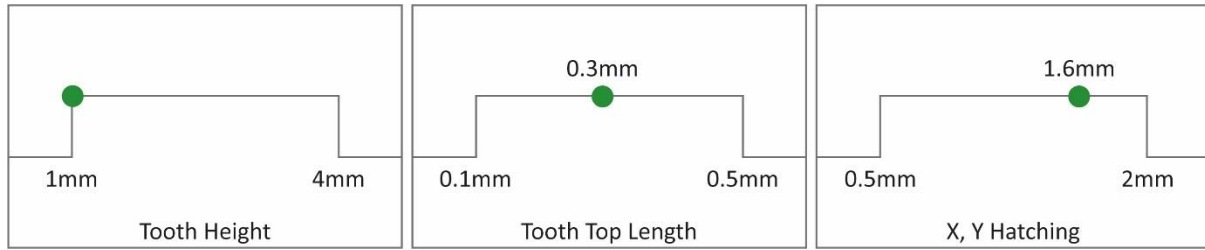
Figure 63. Optimal parameters for block-type supports.
