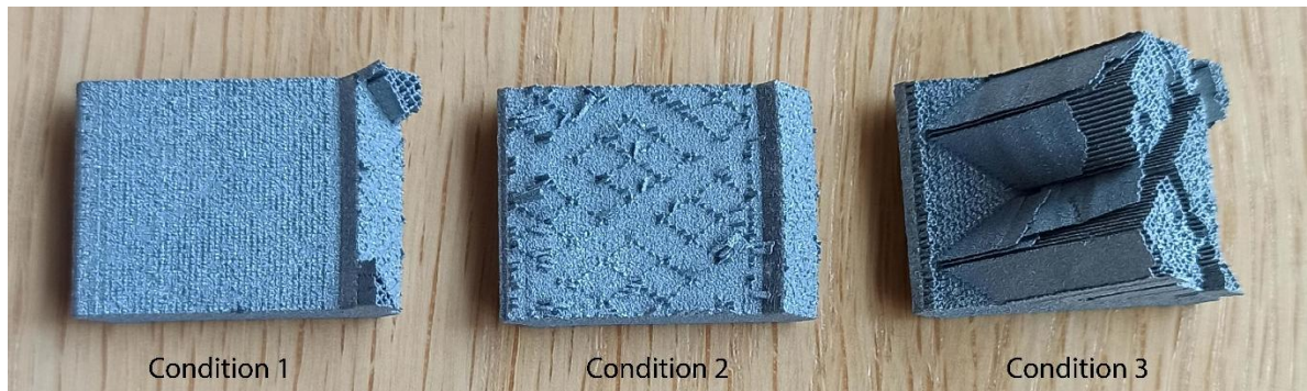
Figure 42. The three conditions of support removability.
