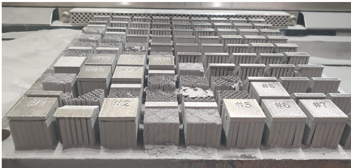
Figure 41. Printed outcome from the SLM machine after removing the unmelted powder.
