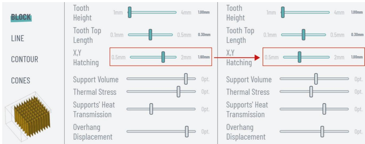
Figure 112. Different optimization outcomes based on 1.6 mm and 1 mm of x, y hatching, respectively.
