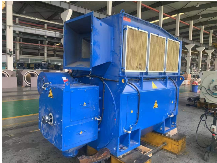
Figure 2.8: Wind turbine generator is the core component responsible for converting the mechanical energy captured by the rotor into electrical energy.
