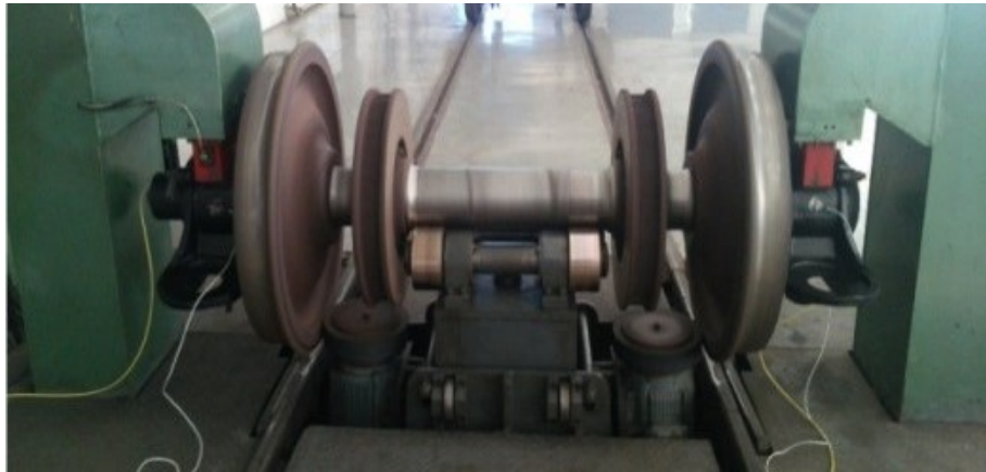
Figure 2.6: Wheelset, is the part of the rolling stock, consists of two wheels on the left and right firmly pressed on the same axle.
