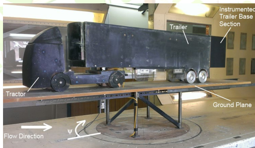
Fig. 1. Wind tunnel test setup with instrument base, Re_n = 8 \times 10^5 .
