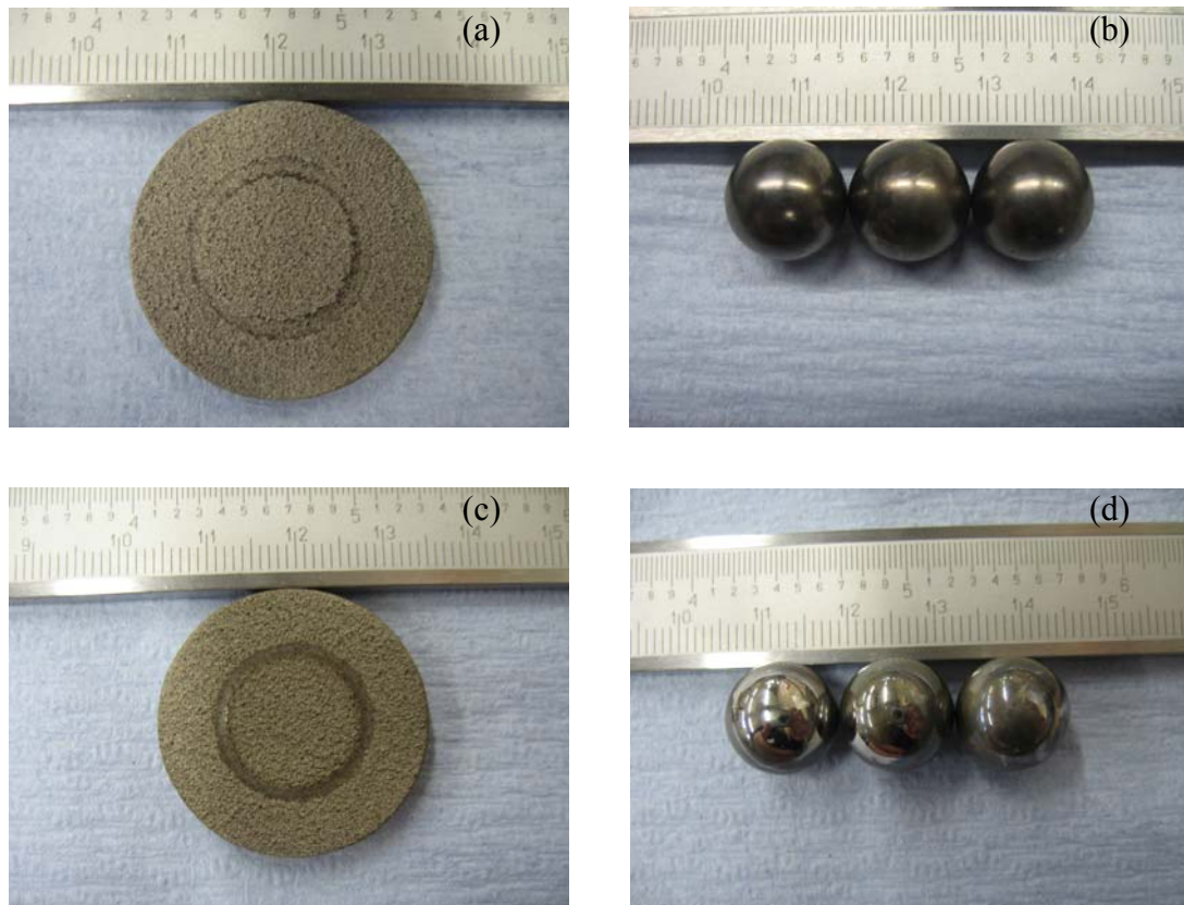
Figure 5.41 Overview of titanium coating disc and balls; (a) and (b) dry conditions, after 37,422 cycles; (c) and (d) seawater conditions, after 149,686 cycles.
