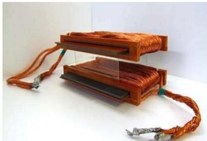
Fig. 2.20 WPT with a flux pipe spiral wound coil [45]
