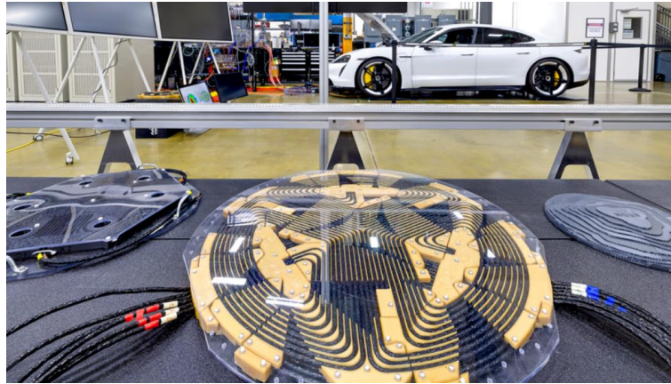
Fig. 2.8 Polyphase 270kW wireless charger [36]
