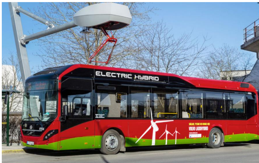
Fig. 2.3 Opportunity Charger where a pantograph delivers power to a bus [15]
