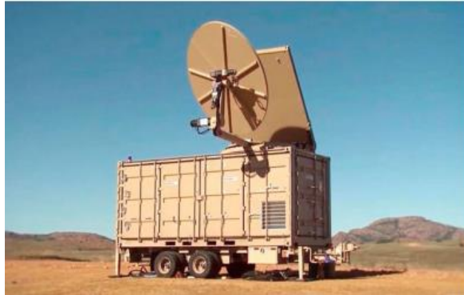
Fig. 2.14 Vehicle mounted microwave WPT system [39]
