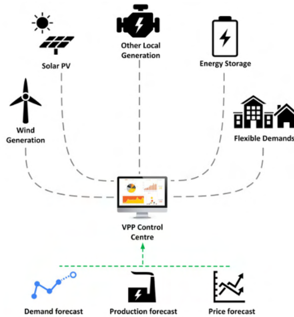
Figure 1.4: A simple schematic of a typical Virtual Power Plant configuration.
