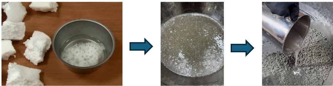
Figure 2 Dissolution of EPS foam in a solvent to form liquid EPS (L-EPS) additive.
