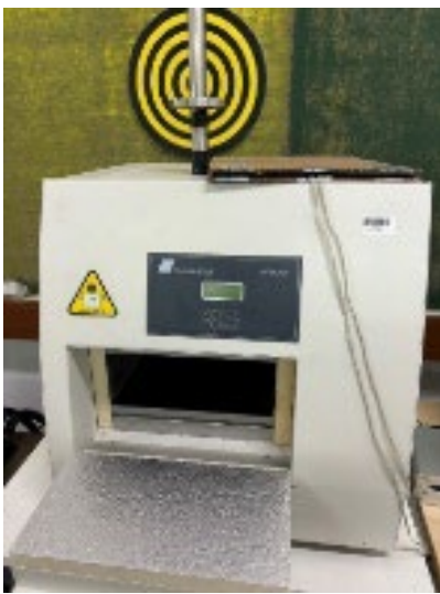
Figure 3a. Guarded-Hot-Plate Apparatus
