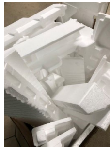
Figure 1a. Recycled Expanded Polystyrene (EPS)
