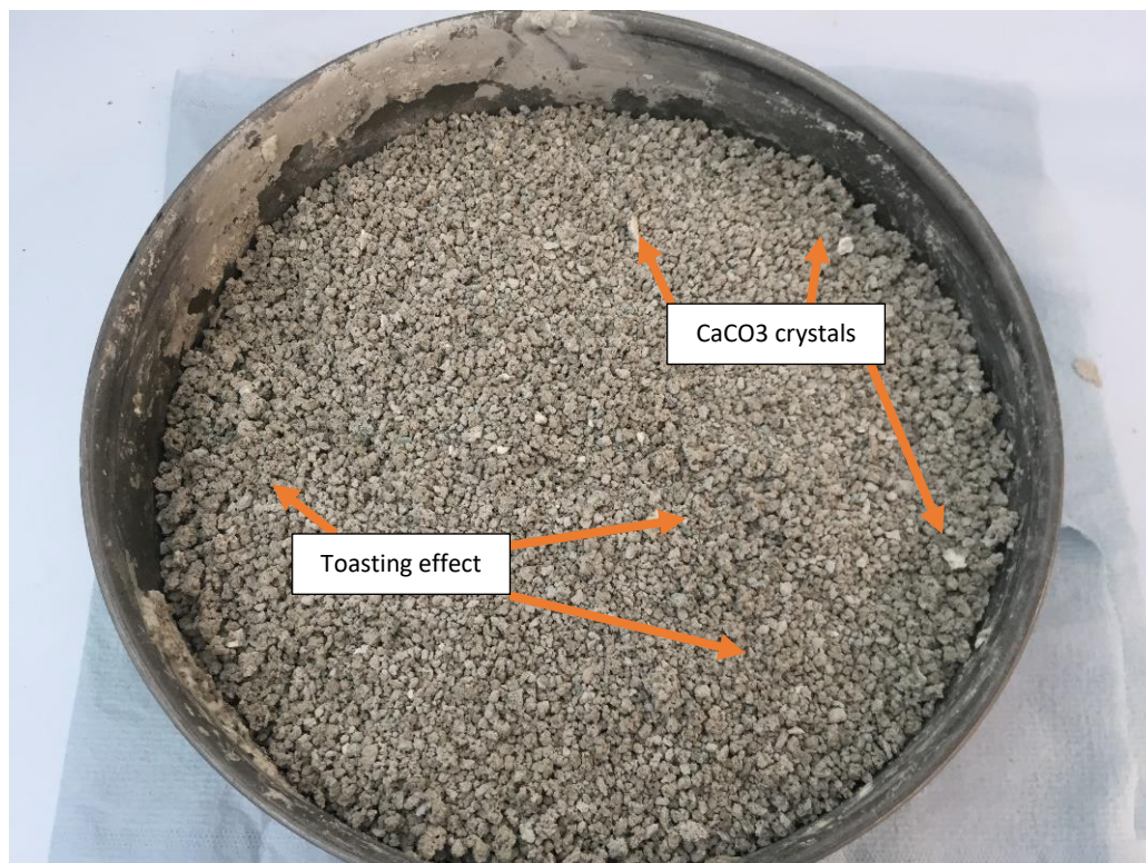
Figure 87 Impregnated AARC particles subject to 24 hours oven drying at 40°C.
