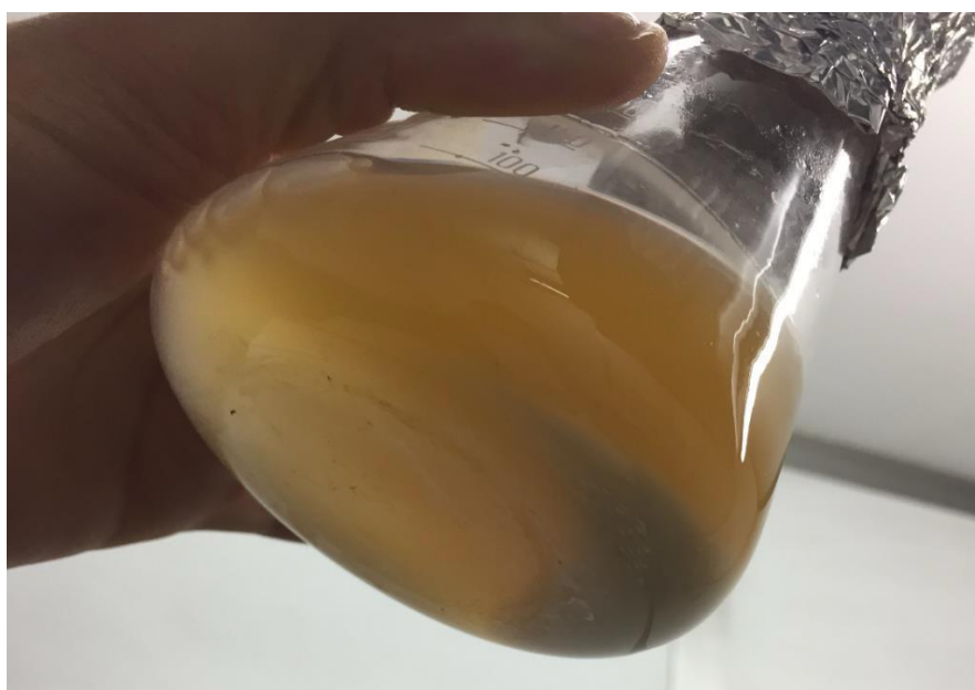
Figure 81 In-vitro calcium carbonate precipitation.
