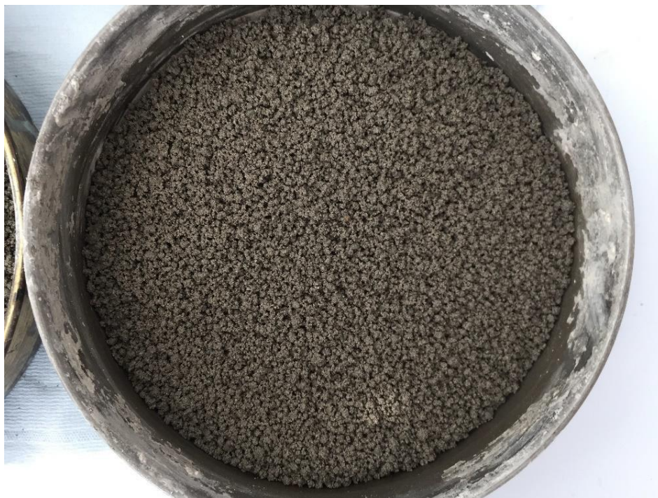
Figure 88 Impregnated AARC aggregates subject to freeze drying.
