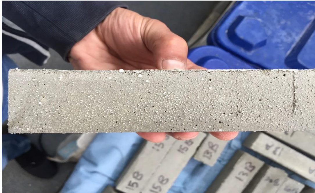
Figure 107 Loss of the calcium carbonate crystals during the wet dry cycle.
