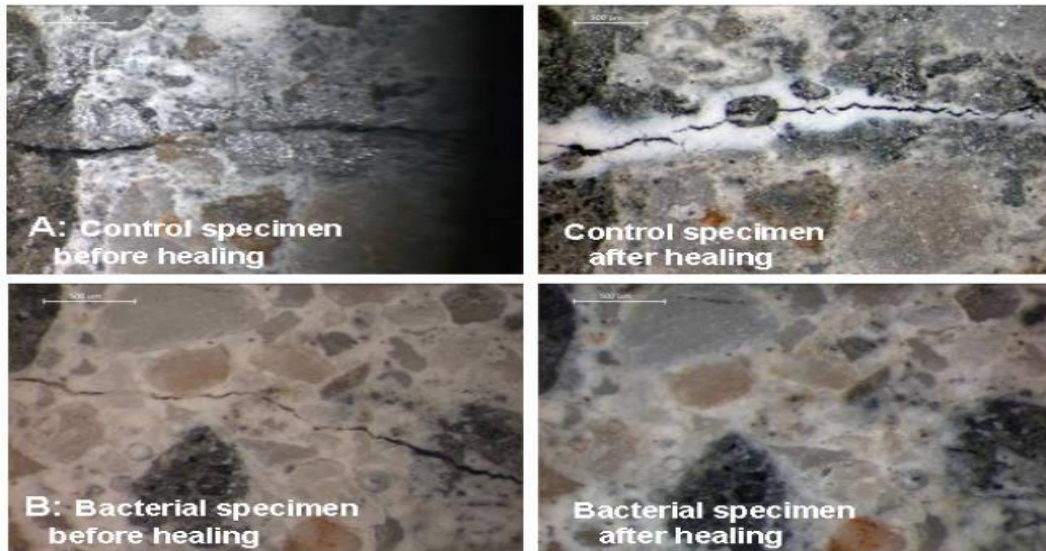
Figure 1 Light microscopic images of pre-cracked concrete in control and bacterial concrete, Jonker et al 2010.
