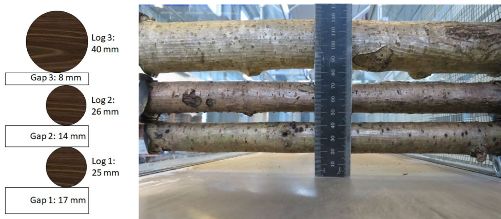
FIGURE 8 | View of the Leaky dams with natural logs (right) and dimensions of logs and gaps (left). Natural-U and Natural-S.
