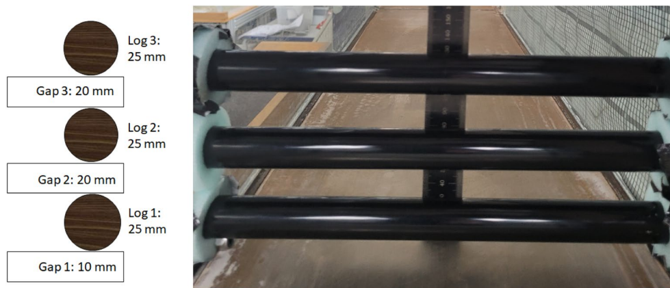
FIGURE 7 | View of the Leaky dams with smooth logs (right) and dimensions of logs and gaps (left). Smooth-U and Smooth-S tests.
