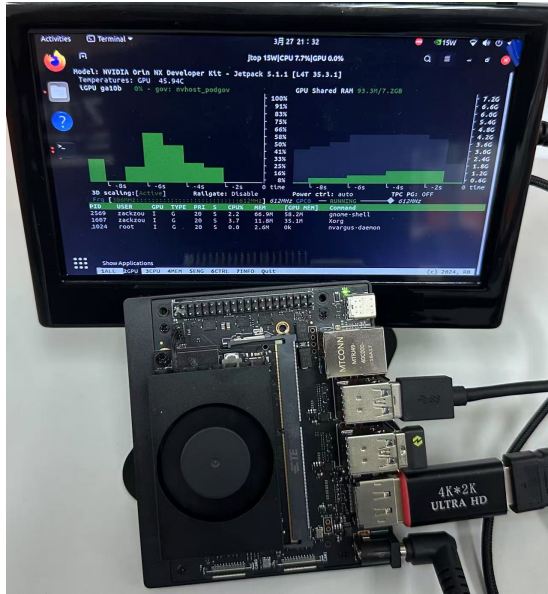
Fig. 5. Schematic diagram of Nvidia Jetson Orin NX 8G Super device.
