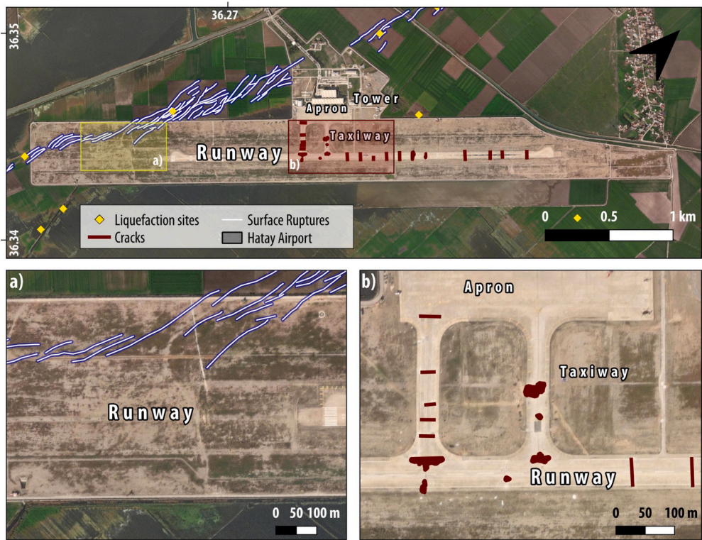
Fig. 11. Satellite view of the HTY airport area. Yellow and red index zones indicate: (a) surface ruptures located on the western side of the runway, and (b) transverse ground cracks and sand ejecta observed along the central and eastern sections of the runway and parts of the taxiway (modified after [86]). (For interpretation of the references to colour in this figure legend, the reader is referred to the web version of this article.)
