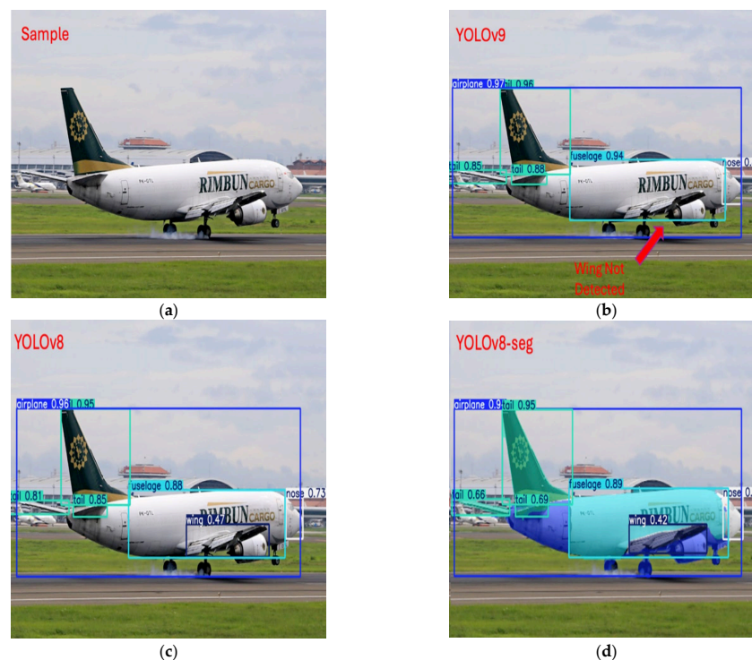
Figure 12. Performance comparison of YOLOv9, YOLOv8, and YOLOv8-Seg under clear visibility conditions, highlighting differences in wing detection and boundary precision: (a) Sample image; (b) YOLOv9 results showing a false negative for the wing class; (c) YOLOv8 predictions with consistent detection across all components; (d) YOLOv8-Seg output combining bounding boxes and segmentation masks for improved interpretability.
