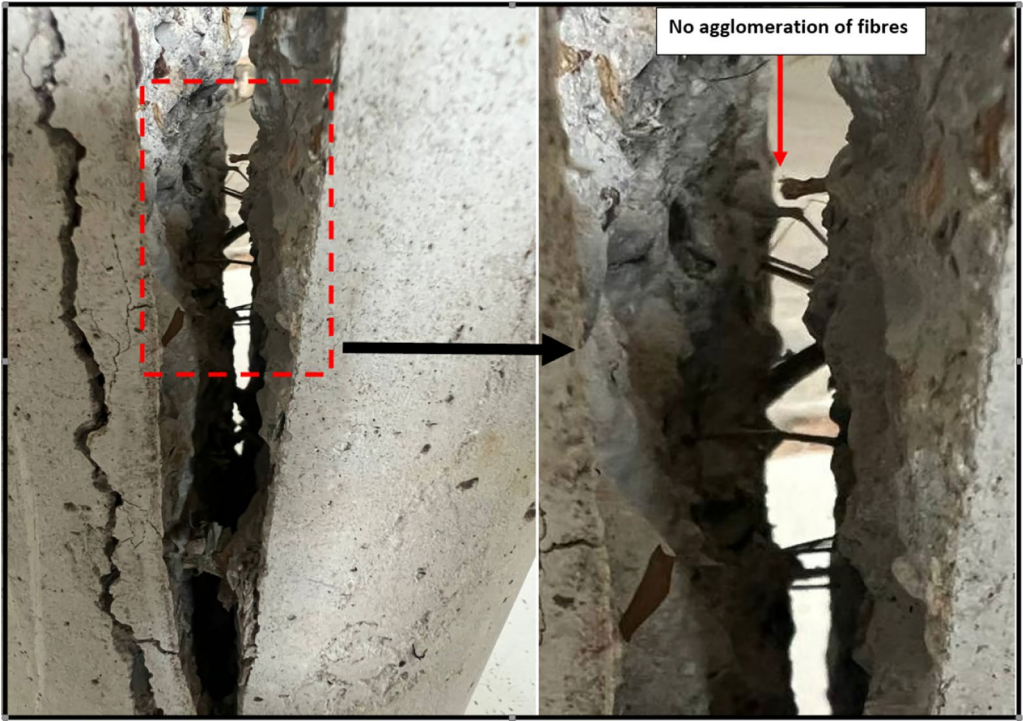
Fig. 9 No agglomeration of PAF at (0.5%), indicating uniform fibre dispersion within the mix
