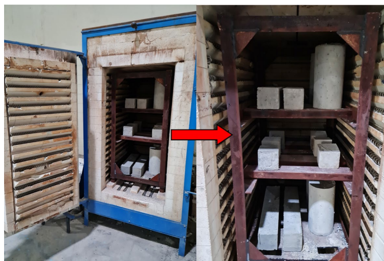
Fig. 2 Electric furnace used for thermal exposure of concrete specimens
