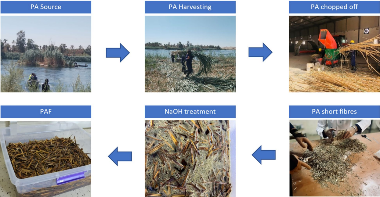
Fig. 1 Process of preparing Phragmites australis fibres (PAF) for concrete reinforcement: from natural harvesting along riverbanks, drying and chopping, to alkaline treatment with NaOH, rinsing, and final drying before incorporation into the concrete mix
