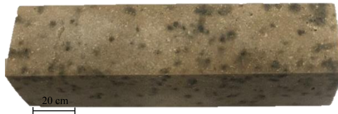
Figure 13. MOC including sawdust, wood fibre and PCM-impregnated aggregates.
