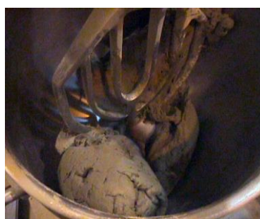
Figure 4. Geopolymer dough-like consistency.
