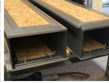
Figure 12. Aluminium profiles with polymer connectors.
