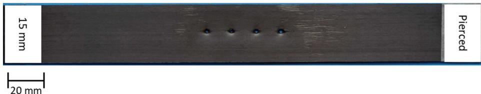
**Figure 4.** Pierced specimens with 15 mm hole spacing prior to OHT testing.
