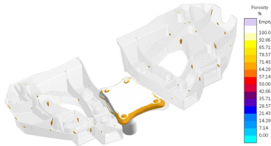
Figure 3 Simulation of casting defects after melt filling and solidification simulation of A356.2 alloy
