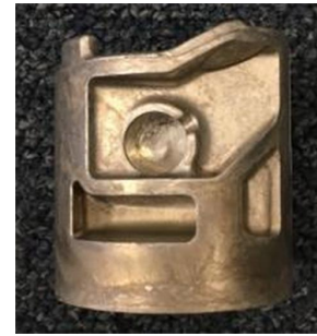
Fig 3. Application of the die-cast Mg 3.5 RE 1.5 GdMnAl alloy for the manufacturing of the piston used in small IC engines.
