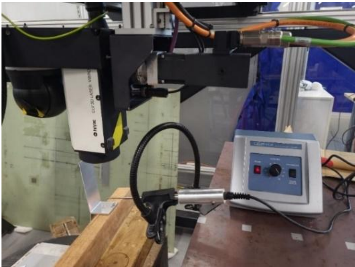
Figure A2. 1: . Experimental setup for vibration analysis during ultrasonic vibration assisted laser welding process
