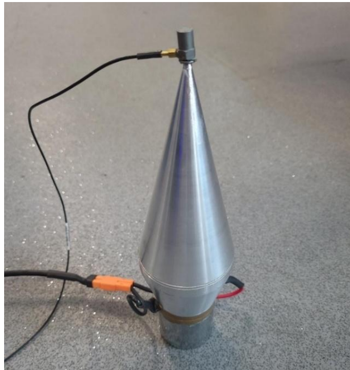
Figure A1. 1: Produced Transducer with a sensor fitted at the tip of the horn
