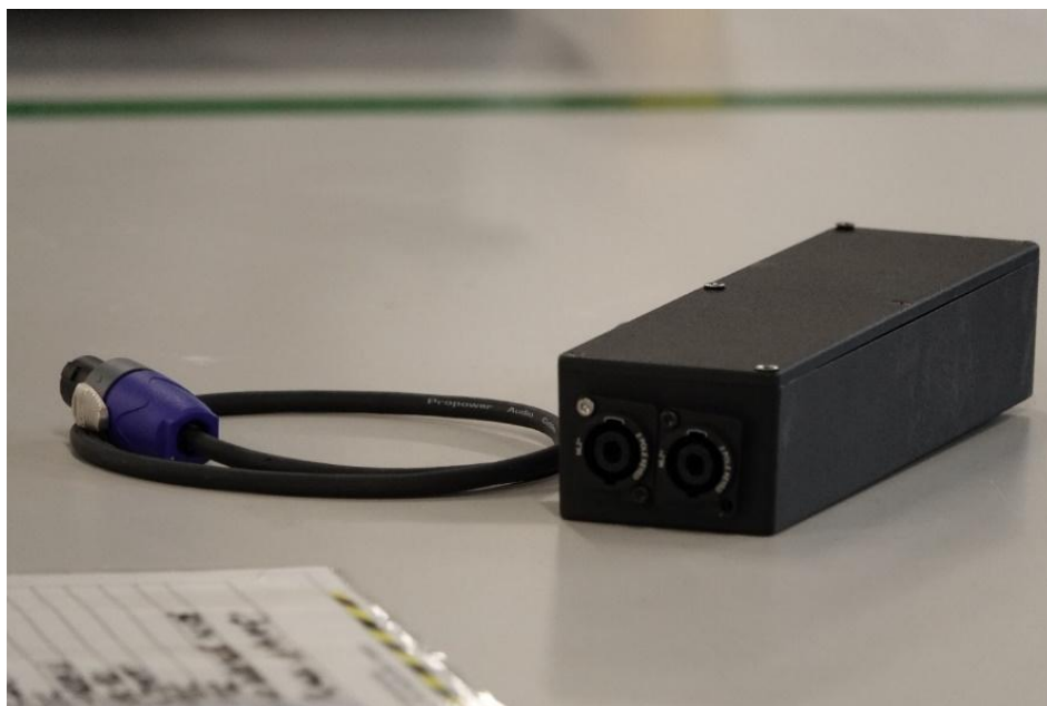
Figure 4. 4: Inline Transformer Unit
