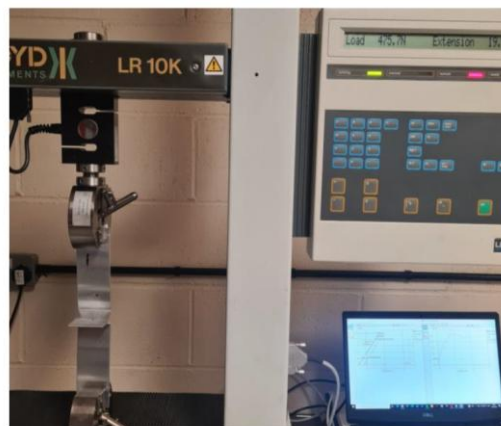
Figure 6. 8: A Lloyd LR10K tensile tester used to conduct pull tests.
