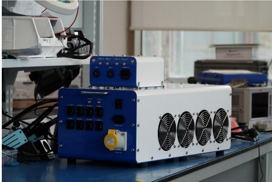
Figure 4. 3: A Complete Ultrasonic Power System
