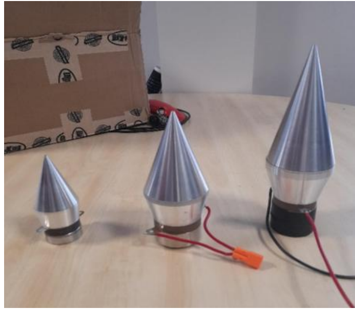
Figure 3. 13: Fabricated Transducers and horns for 20, 28, and 40 kHz.
