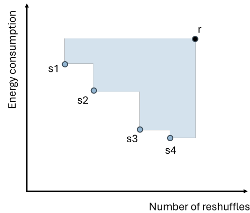
Figure 10. Conceptual illustration of the HV indicator for a bi-objective minimization problem with four hypothetical non-dominated solutions. The reference point r defines the boundary of the dominated objective space.
