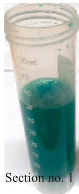
Fig. 17. Typical condensate color in the case of pipe made of Monel 400.
