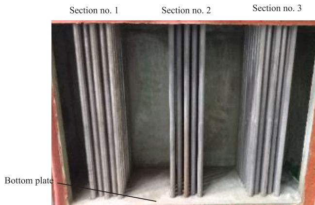
Fig. 18. Internal surfaces of the condensation unit before experiments.
