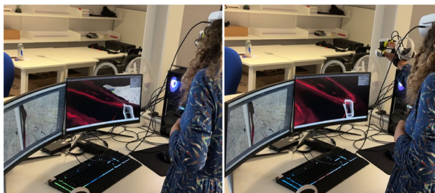
Fig. 7 The system delivers real-time visual rendering and force feedback, enabling the user to perceive cloth deformation and haptic force magnitudes during manipulation
