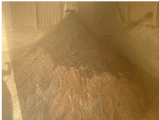
Figure 3. SD was generated during the manufacturing of the wood-wool cement panels.
