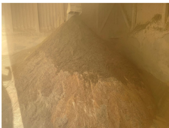
Fig. 3. SD was generated during the manufacturing of the wood-wool cement panels.
