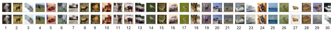
FIGURE 3.7: D-GD reconstruction attack on a line graph consisting of 30 nodes, where the attacker is positioned at one end of the graph. The top row displays the actual inputs for the rest nodes, arranged by their proximity to the attacker, the second row display the output of the attack.
