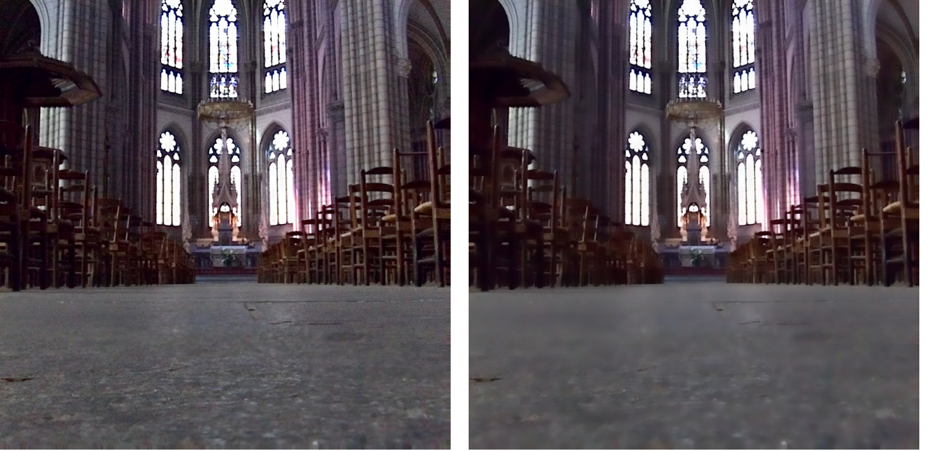
Figure 3.1: Illustration of before and after a guided filter is applied. The left image shows the image that was used as both the guidance image and input image. The right shows the output of the guided filter, where the image has been smoothed, but the edges are preserved.
