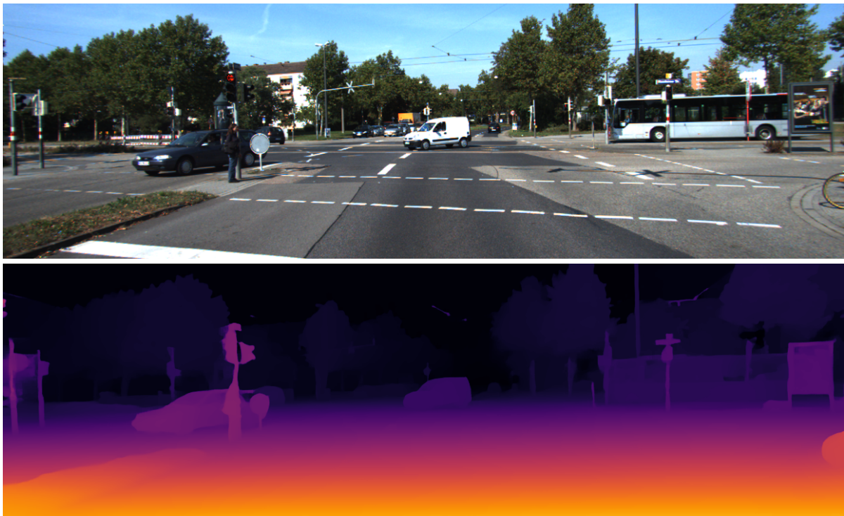
Figure 4.2: The qualitative results from [150] show the top image as the left RGB image from the first example scene from the KITTI-2015 stereo dataset. The corresponding disparity map estimation is shown in the bottom image.
