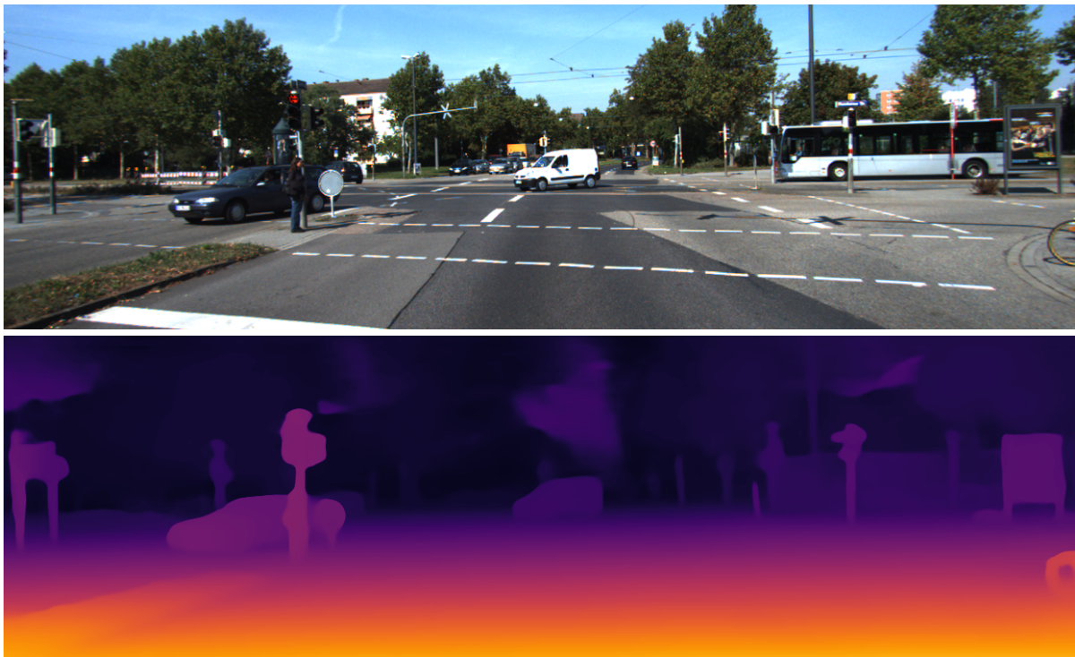
Figure 4.9: The qualitative results from LEAStereo [154] show the top image as the left RGB image from the first example scene from the KITTI-2015 stereo dataset. The corresponding disparity map estimation is shown in the bottom image.
