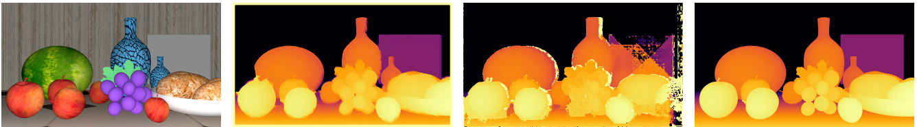
Figure 3.7: Example from the SYNTH3 dataset. From left to right, the first image shows the RGB left stereo rendered image. The second image shows the ToF depth map. The third shows the stereo depth map. The fourth image shows the ground truth depth map.
