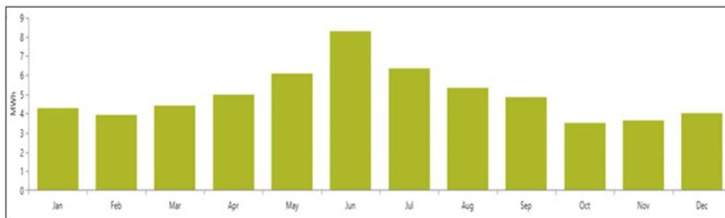
Figure 4.23 Monthly energy production of the wind turbines (@1.5 kg/day)
