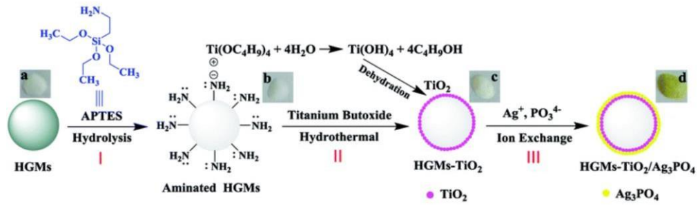
Figure 31. Coating HGMs using a silane coupling agent (An, 2019).
