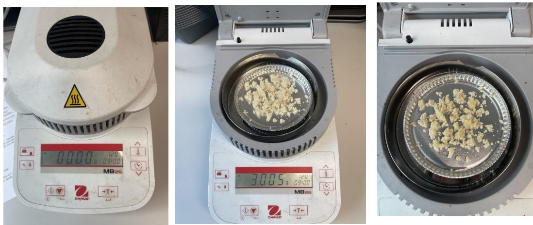
Figure 3.4 Moisture analyser for measuring moisture content
