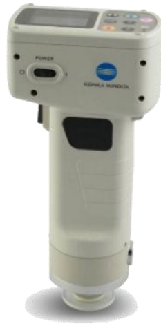
Figure 3.5 Chromameter for measuring colour values
