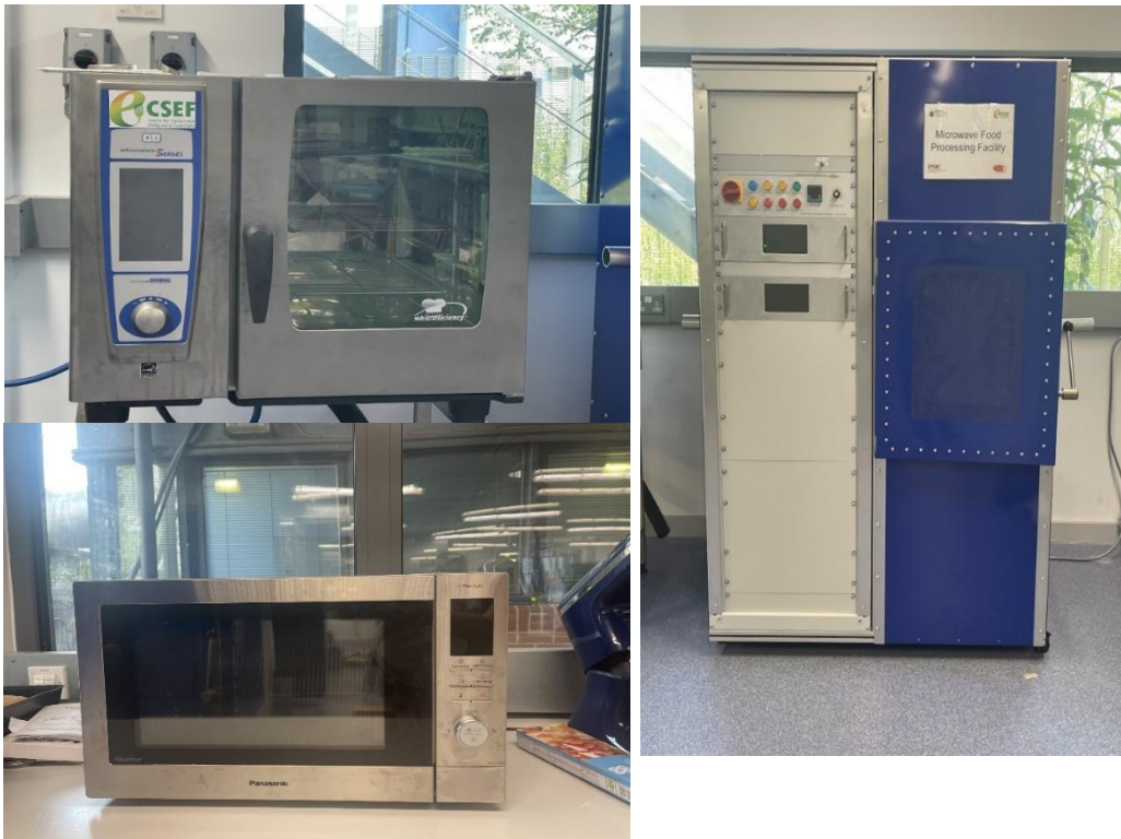
Figure 3.2 The equipment used for different baking modes a) Conventional oven b) domestic microwave and c) industrial solid-state microwave
