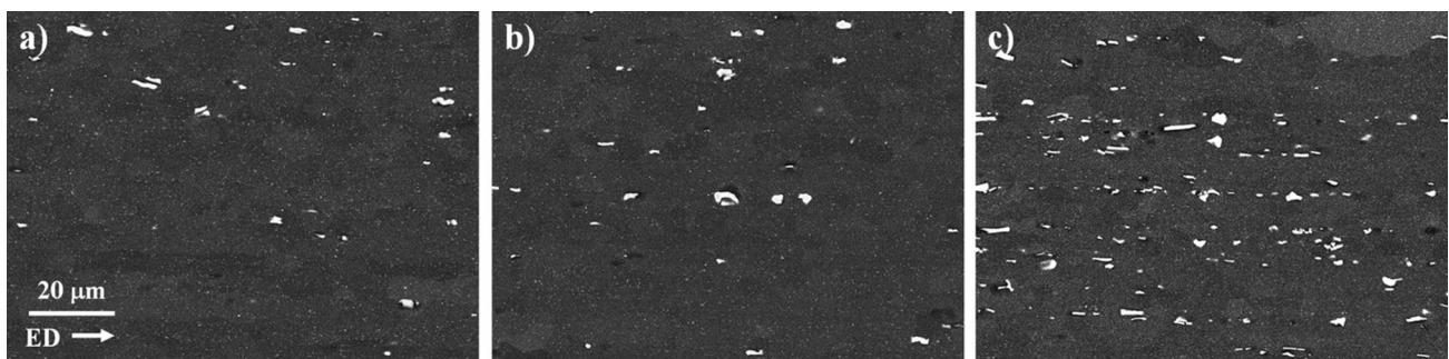
Fig. 3 SEM/BSE images taken at the same magnification at a 0.2Fe, b 0.3Fe, and c 0.5Fe content accompanied by histogram of corresponding area fraction
