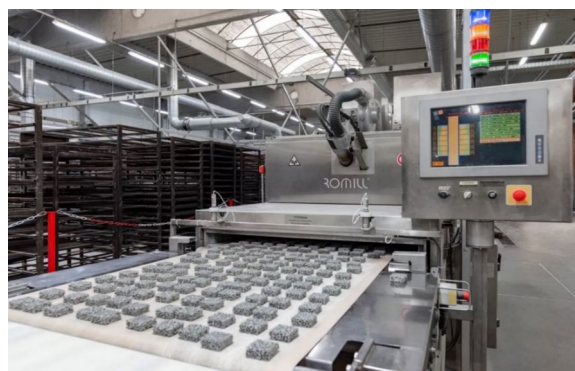
Figure 5: Microwave conveyer belt drying system for drying ceramic foams [6].
