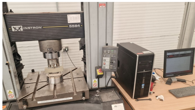
Figure 1. Flexure strength test setup.
