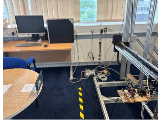
Figure 1 The Prototype of Automated Millimeter Wave Imaging System (center frequency of 76.5 GHz), ensuring half-wavelength spatial sampling. At each scanning position, 256 ADC samples were acquired with a sampling rate of 10 MHz.
