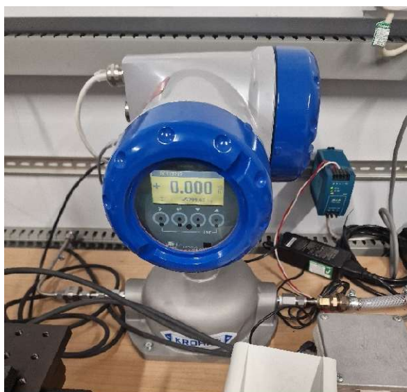
Figure 3.4. Krohne Optimass 3000-S01 Coriolis flow meter and Krohne MFC 300 signal converter for mass flowmeters.
