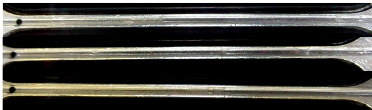
Slug Flow ( G = 58 \text{ kg/m}^2\text{s} , x = 0.48 )
