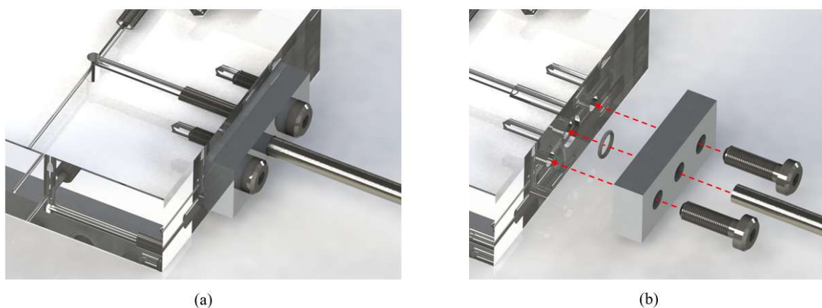
Figure 3.23. Sealing methodology for stainless steel pipework in the test section.
