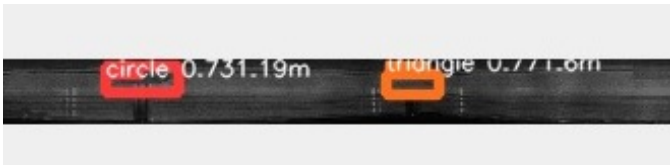
Fig. 5. Detected landmarks (shapes) in environment (in our lab). The detected landmarks are classified with some confidence.
