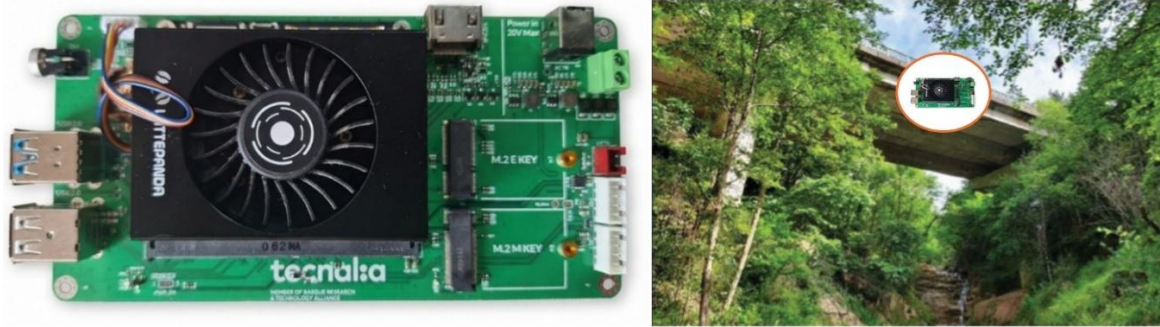
Fig. 5. A custom made (Tecnalia) Edge Computing board with LattePanda MU processor board
