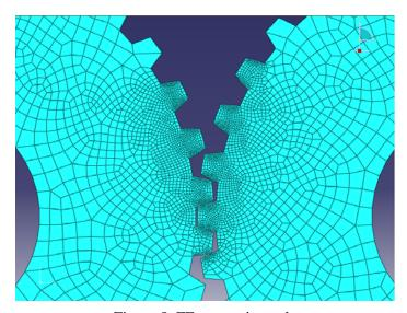
Figure 5: FE gear pair mesh
