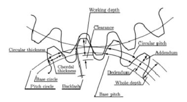
Figure 1: Spur gear nomenclature
