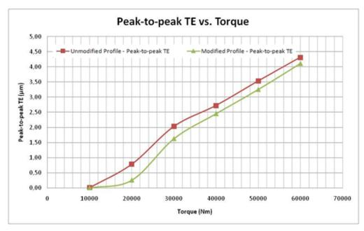
Figure 10: Comparison of peak-to-peak TE for various loads between modified and unmodified profile
