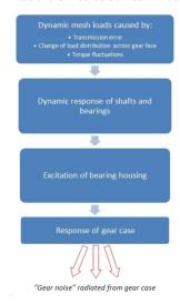
Figure 3: Noise transmission path
