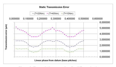
Figure 8: Transmission error plots for different loads
