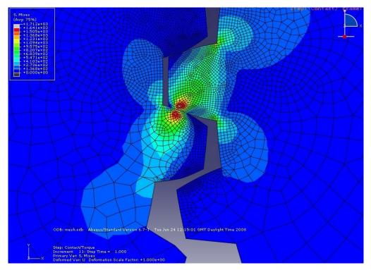
Figure 7: FE gear contact analysis
