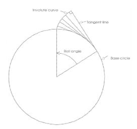
Figure 4: Generation of an involute curve
