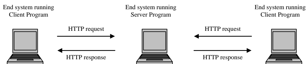
Figure 18: Communication between client and server programs
