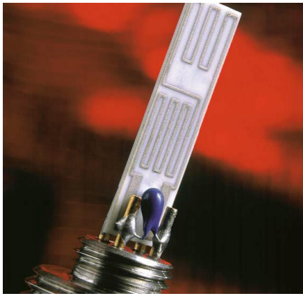
Figure 3-7 TD 2 sensor is an aluminium oxide sensor Michell series 2000 (Michell instrument user guide)
