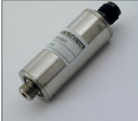
Figure 3-10: The pressure transducer Sensor Technics series CTE8000 used in the mass flow-mixing generator.
