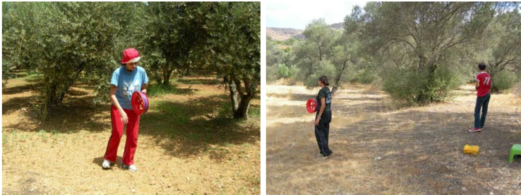
Fig. 4.27: TEM data acquisition in Geropotamos study area. At the two lower photos, the two participants set the antenna (50 x 50 m square).
