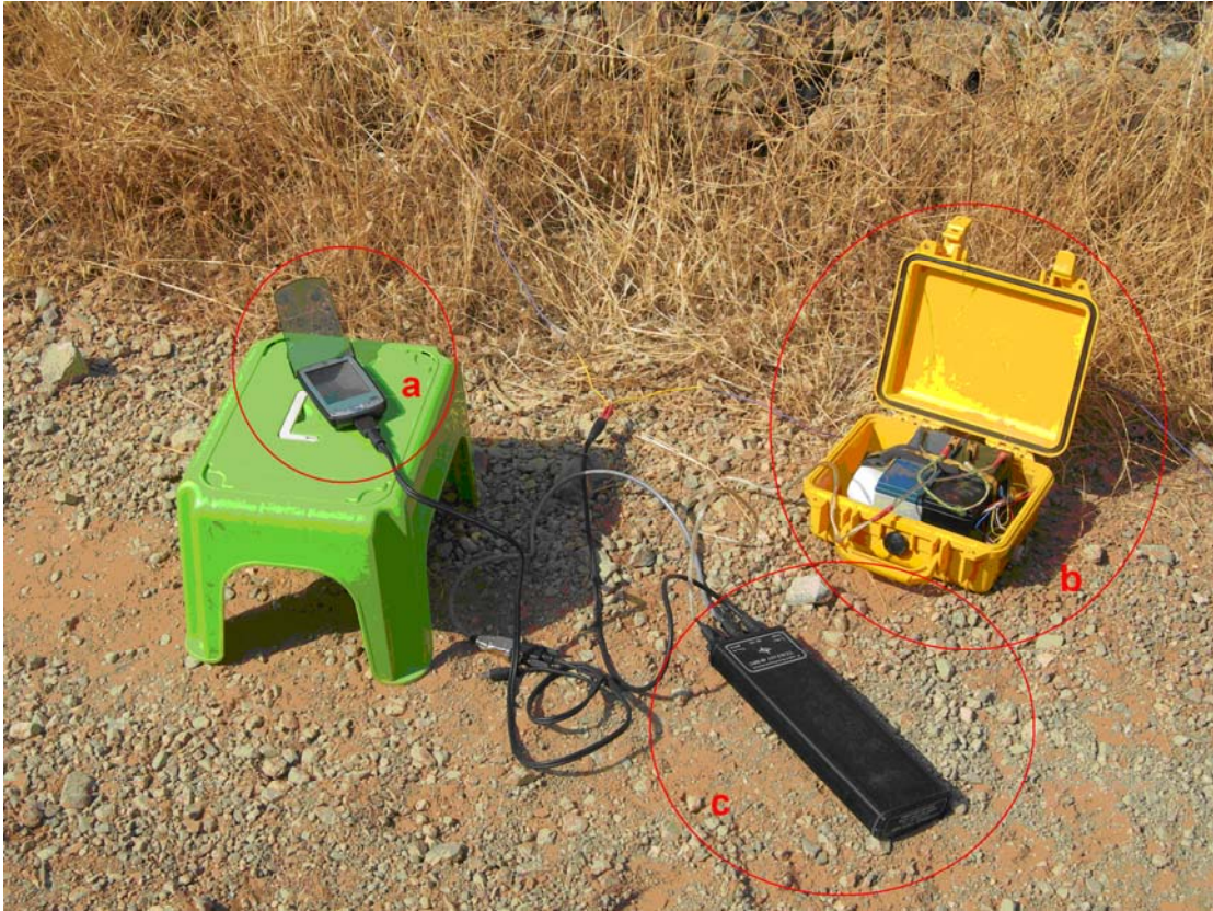
Fig. 3.8: TEM instrumentation and peripheral units: a) palmtop PC, b) external power supply (12V+12V in series =24V), c) TEM Fast 48 system
