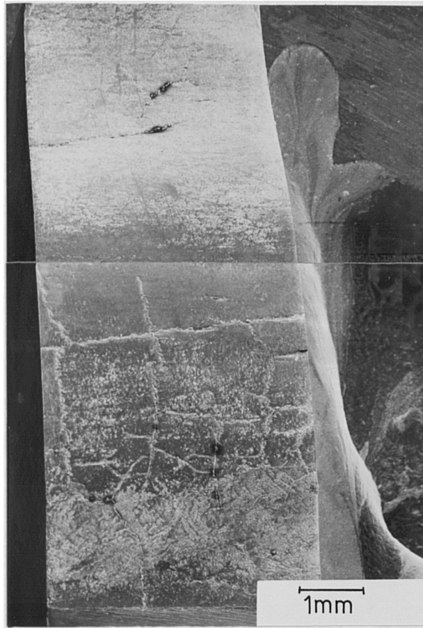
Figure 4.3.35. Chieftain gun barrel. Bore surface in the region of "commencement-of-rifling".
